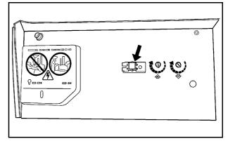
2. Locate in the garage, the garage door opener receiver (motor-head unit). Locate the "Learn" or "Smart" button. It can usually be found where the hanging antenna wire is attached to the motor-head unit and may be a colored button. Press this button. After pressing this button, complete the following steps in less than 30 seconds.
